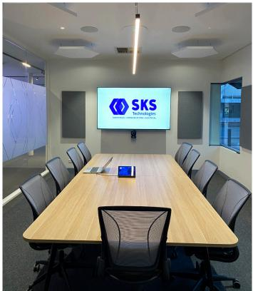
To further enhance the audio environment, the available wall spaces were fitted with Broadway B4848–SQ2 Square–Edged panels in a grey finish. These panels not only complemented the room's aesthetics but also played a crucial role in dampening the problematic audio reflections.
