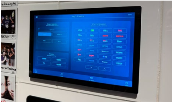
A RTI IST-10 10-inch touchscreens hosts the WED Group-designed UI. Matthew Joyce: "Thanks to the RTI control, managing the AV, especially the TVs, is now very straightforward for the club. You're not reliant on a tech-savvy staff member to figure things out – it's easy."
